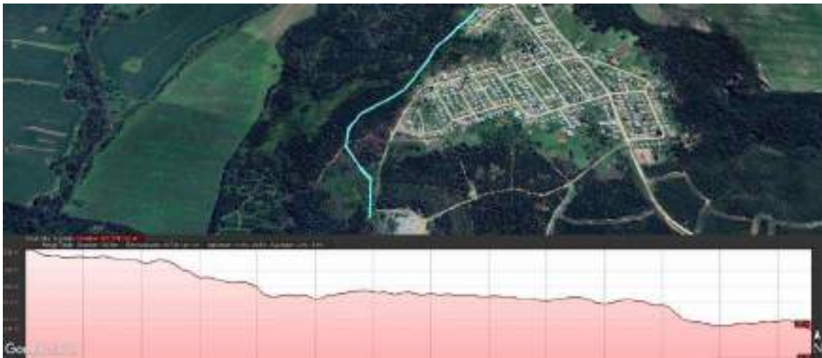
Figure 24: General gradient of Pipeline – alternative 1
