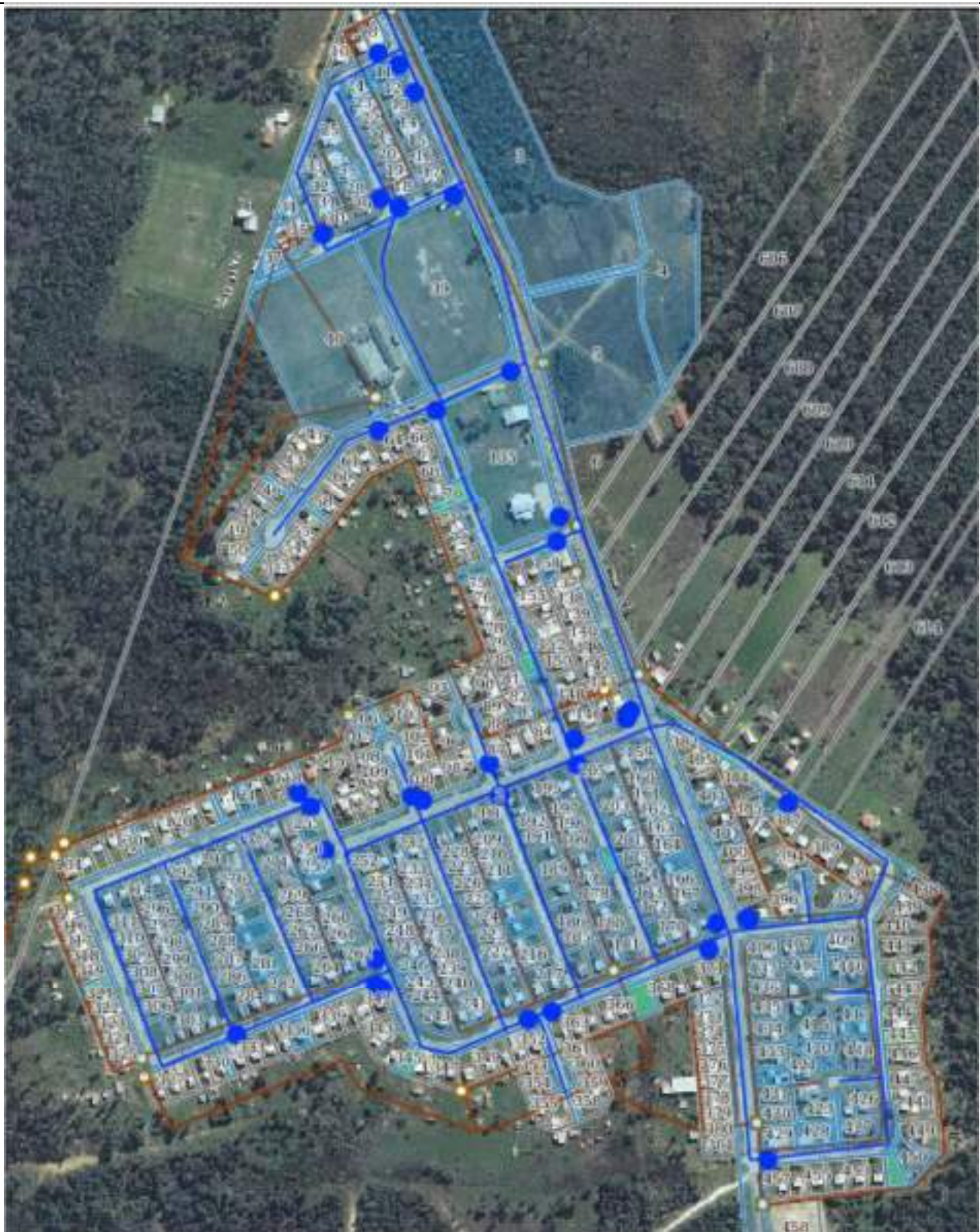
Figure 3: Existing Sewer Reticulation, Woodlands Settlement (SMEC, July 2025)
