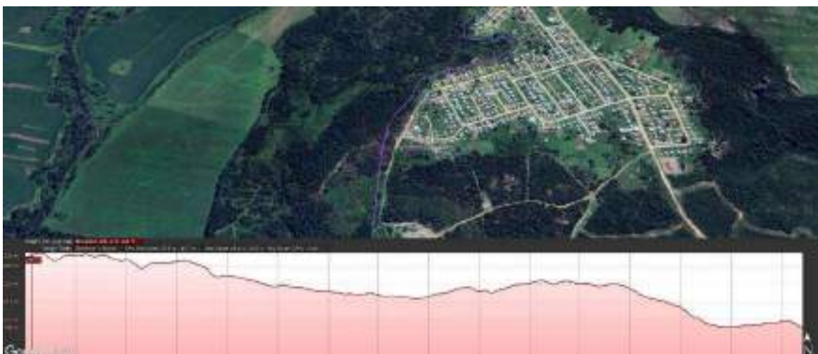
Figure 25: General gradient of Pipeline – alternative 2
