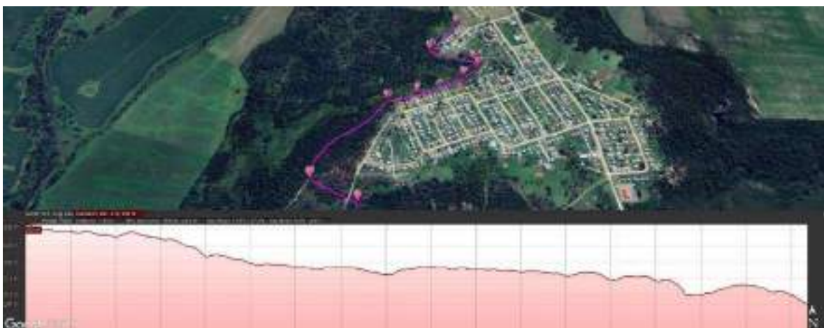
Figure 26: General gradient of Pipeline – alternative 3
