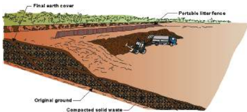
Figure 10: Illustration of the area method of sludge co-disposal on landfill
