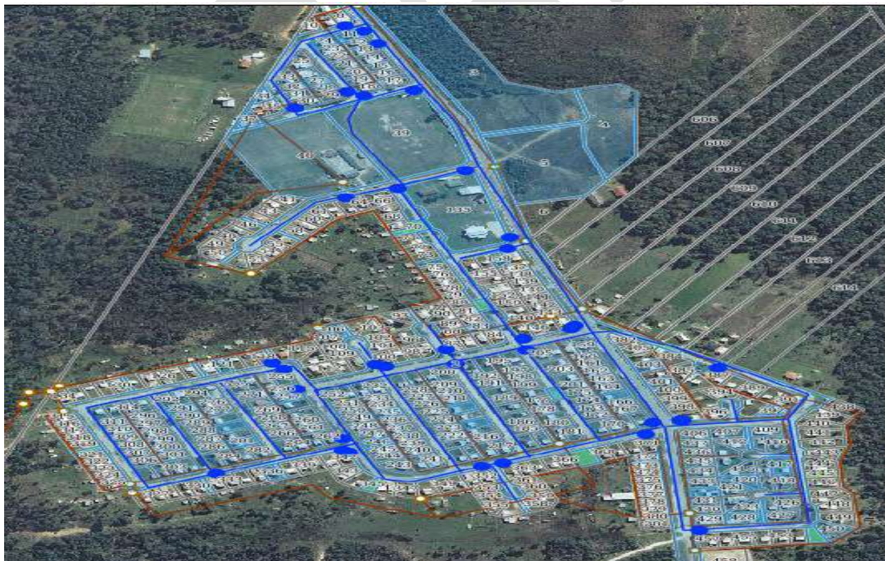
Figure 4-6 Existing Sewer Reticulation
