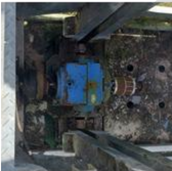
Figure D Corroded Motor
